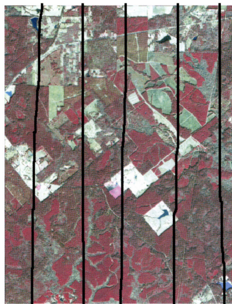
Fig. 2 Parallel transects flown by a profiling LiDAR (profiler) over a study site: the dark lines are the flight lines of the laser profiler, the background is a false-color QuickBird image.
