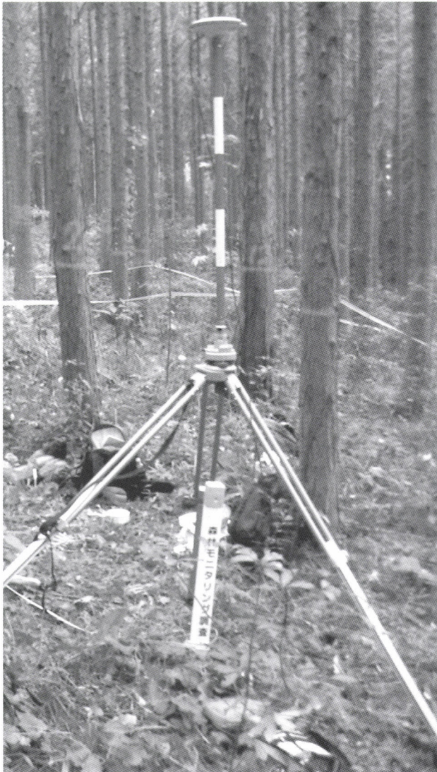
Fig. 2 The high-precision, dual-frequency carrier-phase GPS used in the present study (GSR-2600, SOKKIA).
