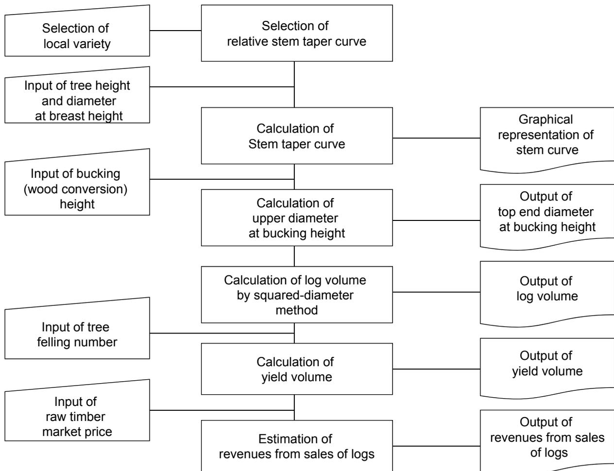
Fig. 3 Flow chart of forest operation planning based on stem upper diameter estimation
