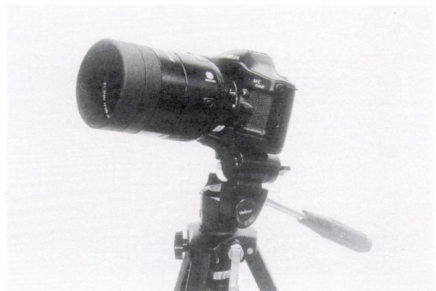
Fig. 1 The measuring camera MC-100
